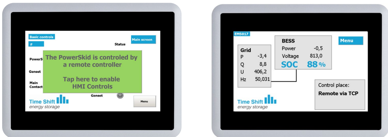
Figure 33: Example of HMI views informing the operator about the control place
