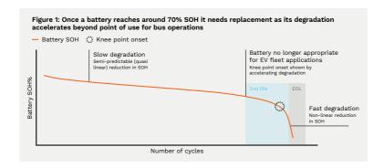
Ultimately, under expected degradation rates, heavy-duty fleet batteries will need to be replaced at least once in a fleet vehicle's life.
