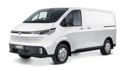
Range/Battery: 218km/77 or 88kWh Body: SWB, LWB, LWB high roof
